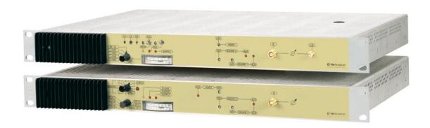
The radio links on 23 Ghz are composed by two units; an indoor unit (IDU) supplied in a single 1-unit rack containing the mo/demodulator stage, and an outdoor unit (ODU) in aerial head containing SHF part.
