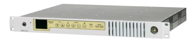
The radio links are composed by two units; an indoor unit SHF (IDUSHF) (optionally outdoor unit ODU in aerial head) supplied in a single 1-unit rack containing the RF Transmitter (or RF Receiver) and a second indoor unit LF (IDU-LF) supplied in a single 1-unit rack containing mo/demodulator (QPSK or 16QAM MO/DEM) and co/decoder (MPEG2 CO/DEC + MUX).
