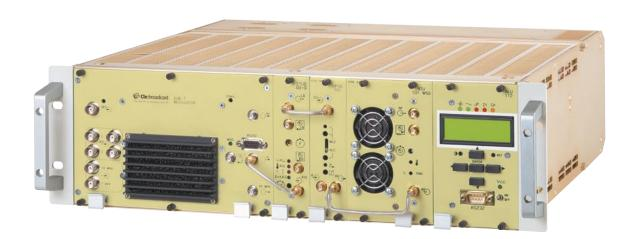
Compliant with ETS 300 744 requirements Channel Bandwidth 6, 7, 8 MHz all uniform DVB-H support thanks to 4k IFFT mode, Cell-id and 8k symbol interleaver Superior linear and non linear digital pre-corrector. Dual ASI for each input (LP & HP) MIP decoder for automatic configuration De-jitter on input signal prior to transmission GPS reference lock signal Superior MER performance (designed to meet 45 dB) All redundancy configurations available on request (Dual driver; active reserve; N+1; 1+1)
